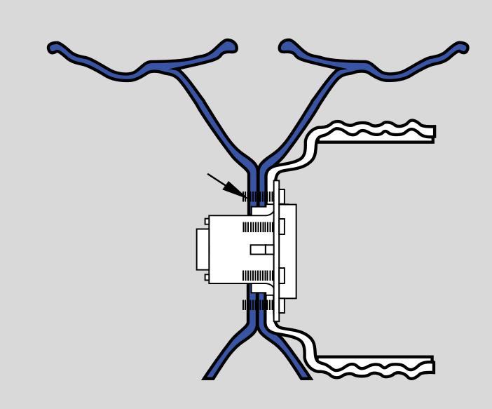
Apply two drops of oil on leading threads of studs and between nut body and flange. Avoid getting oil on face of nut, wheels, or brake drum.
