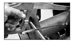
6 The pushrod should be cut to the proper length. Follow the installation instructions for the ABA using the ABA installation guide. You can now un-cage the spring brake.
