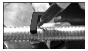
**6** Remove both the black pushrod cutoff tool and ABA installation guide. Cut the pushrod perpendicular to the mark.
