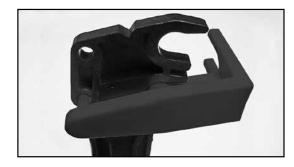
Install the ABA installation guide over the S-cam and position the notch in the black pushrod cutoff tool on the pushrod. Make sure the ABA installation guide is parallel and centered on the pushrod.
