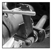
The pushrod should be parallel with black pushrod cutoff tool, NOT at an angle. If it is at an angle, the arm length or chamber mounting are incorrect. Mark the pushrod in front of the black tool.
